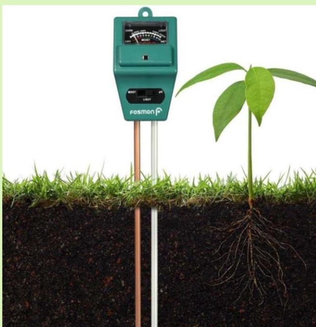
Figure 3. Probe that measures the pH in the soil (Bibli, n.d.)
