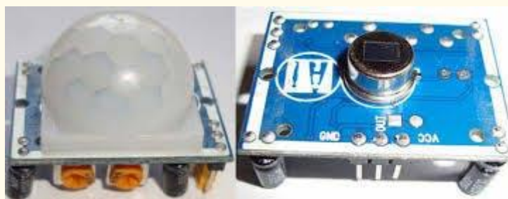
Figure 1 PIR Sensor, source: https://create.arduino.cc/projecthub/biharilifehacker/arduino-with-pir-motion-sensor-fd540a
