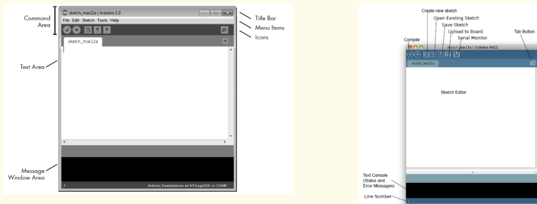
Figure 9 The Arduino IDE on Windows (picture on the left, source: Boxall, 2013), and Mac (picture on the right, source: Smith, 2011).
